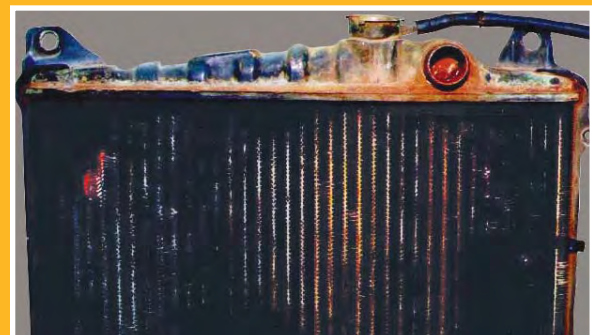
If the Radiator is Neglected, Rust and Corrosion Can Form, Causing Leaks and System Failure
