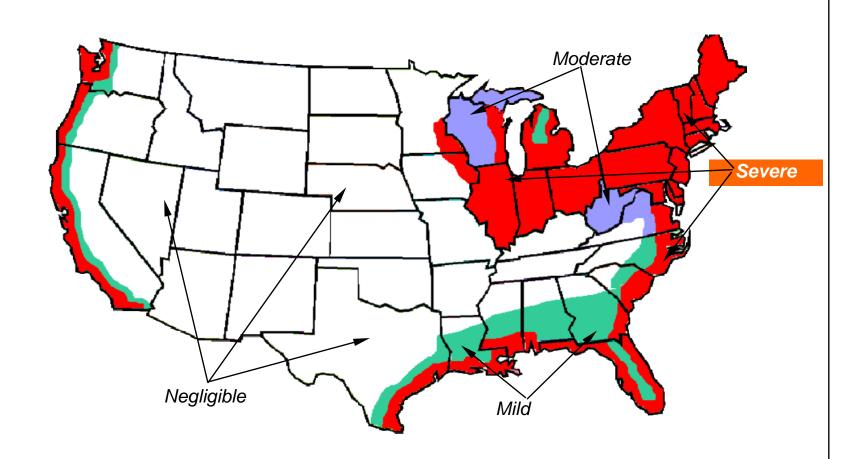
"Corrosion Zones" identify areas with environmental factors that accelerate the formation of corrosion due to weather conditions and industrial contaminants.
