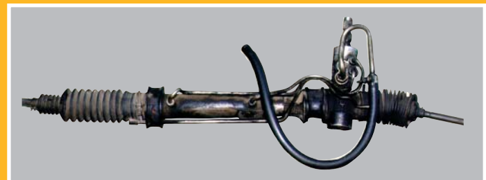
If Not Properly Serviced, the Power-Steering Unit Can Wear Out, Degrading Performance
