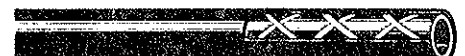
SAE J844 Type B Extruded Nylon inner tube, one layer of open ply fiber reinforcement and a Nylon outer cover. (3/8", 1/2")
